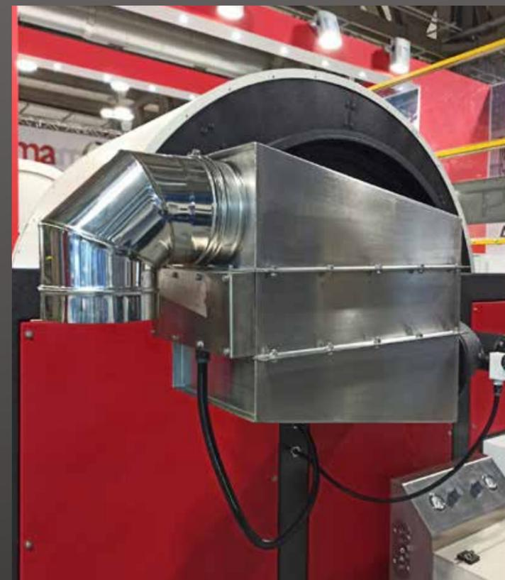
SISTEMA DI RISCALDAMENTO A RESISTENZE ELETTRICHE
