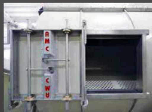
PARTICOLARE DELLA PORTA SCORREVOLE IN ACCIAIO INOX 316L RIVESTITA IN POLIPROPILENE
